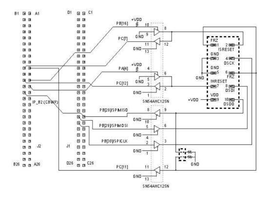
When the BDM handler board is plugged and the BDM connector is left un-connected, the two jumpers should be installed. In this case, the input values read on the pins PC[28]/SPIMISO, PC[10], PC[7], PC[6], are all logical '0'.
